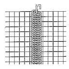
The vertical joints of adjacent units are connected by inter-linking vertical joining coils and inserting a locking pin, front and rear of the Trapions. The horizontal joining coils connecting the lid should be positioned at the front of the trapion.
