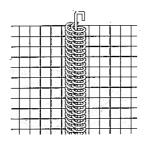
The vertical joints of adjacent units are connected by inter-linking vertical joining coils and inserting a locking pin, front and rear of the gabions. The horizontal joining coils connecting the lid should be positioned at the front of the gabion.
