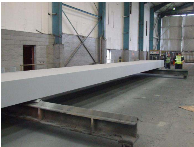
One of the 20-ton zingaised beams being checked
