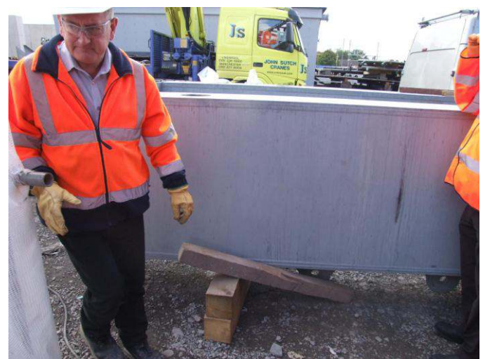
Checking the zinc-thickness on the zinganised beams
